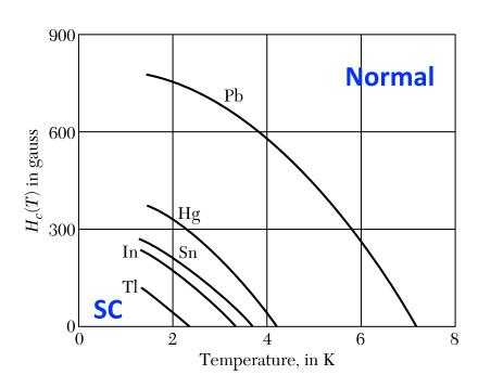
If the magnetic field strength  $H_{\rm ext}$  is further increased, then at a critical field strength  $H_{\rm c}$  it is energetically more favorable for the material to convert to the normally conducting phase, in which the magnetic field penetrates the material. The phase boundary between superconducting and normally conducting states corresponds to the critical magnetic field  $H_{\rm c}$  (T).
