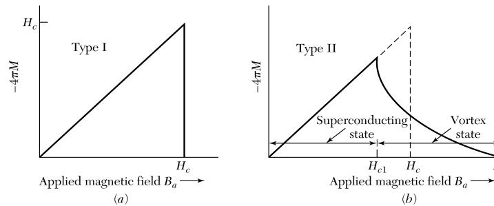
Pure specimens of many materials exhibit this behavior; they are called type I superconductors or, formerly, soft superconductors. The values of  $H_c$  are always too low for type I superconductors to have application in coils for superconducting magnets.
