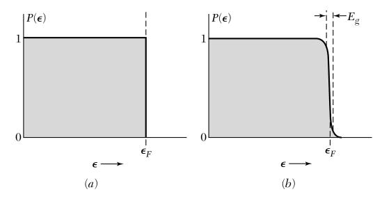
The central feature of the BCS state is that the one-particle orbitals are occupied in pairs: if an orbital with wavevector  $\mathbf{k}$  and spin up is occupied, then the orbital with wavevector  $-\mathbf{k}$  and spin down is also occupied. If  $\mathbf{k} \uparrow$  is vacant, then- $\mathbf{k} \downarrow$  is also vacant. The pairs are called **Cooper pairs** and have spin zero as well as many attributes of bosons.
