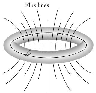
The flux through the ring is the sum of the flux  $\Phi_{ext}$  from external sources and the flux  $\Phi_{sc}$  from the superconducting currents which flow in the surface of the ring;
