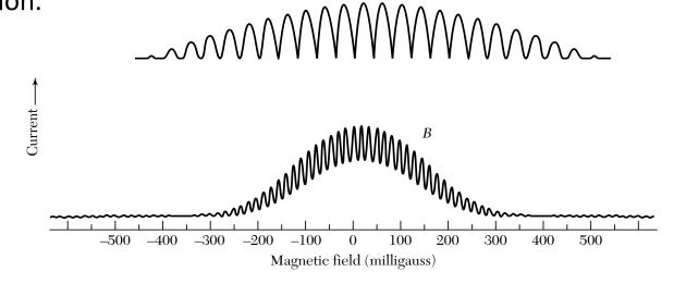
The field periodicity is 39.5 and 16 mG for A and B, respectively. Approximate maximum currents are 1 mA (A) and 0.5 mA (B). The junction separation is 3 mm and junction width 0.5 mm for both cases. The zero offset of A is due to a background magnetic field.
