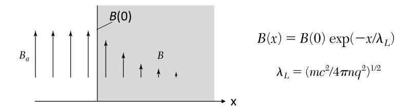
An applied magnetic field  $\mathbf{B}_a$  will penetrate a thin film fairly uniformly if the thickness is much less than  $\lambda_L$ ; thus in a thin film the Meissner effect is not complete. In a thin film the induced field is much less than  $\mathbf{B}_a$ , and there is little effect of  $\mathbf{B}_a$ . It follows that the critical field  $\mathbf{H}_c$  of thin films in parallel magnetic fields will be very high.
