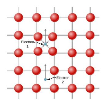
An electron moving through a conductor will attract nearby positive charges in the lattice. This deformation of the lattice causes another electron, with opposite spin, to move into the region of higher positive charge density. The two electrons then become correlated. Because there are a lot of such electron pairs in a superconductor, these pairs overlap very strongly and form a highly collective condensate.
