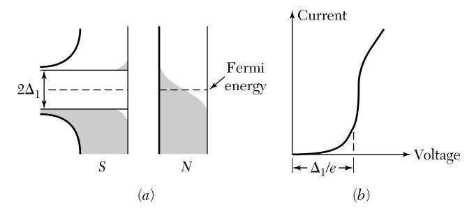
The density of states and the current-voltage characteristic for a tunneling junction.
