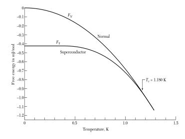
The free energy density  $F_N$  of a nonmagnetic normal metal is approximately independent of the intensity of the applied magnetic field  $\mathbf{B}_a$ . At a temperature  $T < T_c$  the metal is a superconductor in zero magnetic field, so that  $F_s(T, 0)$  is lower than  $F_N(T, 0)$  by
