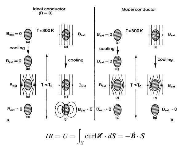
Vanishing resistance implies that the magnetic flux  $\mathbf{B} \cdot \mathbf{S}$  through the closed loop may not alter after cooling and after switching off the external field  $\mathbf{B}_{\text{ext}}$ .
