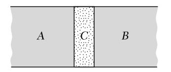
Two metals, A and B, separated by a thin layer of an insulator  $C \sim 10 \text{ Å}$ .
