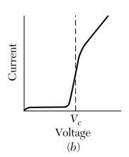
(a) Linear current-voltage relation for junction of normal metals separated by oxide layer; (b) current-voltage relation with one metal normal and the other metal superconducting.
